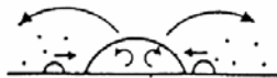
Fig. 9. Behaviour of the particles at higher acceleration. Ejection of particles and formation of secondary hills followed by reunification. On the bottom the simplified model is represented
